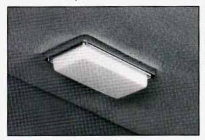
The dome lamps may come on when you open any of the doors. You can also turn on the dome lamps by turning the dimmer dial clockwise until it clicks.
